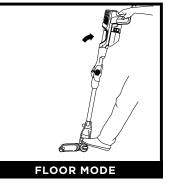
To clean floors, place foot on floor nozzle and tilt handheld vacuum back.
