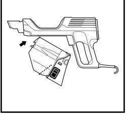
To reinsert the dust cup back into the handvac, angle the tip first and then push up until it clicks into place.
