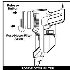
Remove the filter cover on the top of the handvac to access the post-motor filter. The **Post-Motor Filter** should be washed once every 9 months.
