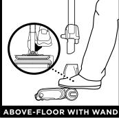
Detach the wand for more reach to clean ceilings, skirting boards, window sills, and other hard-to-access areas. To disconnect the wand, stand the vacuum upright. Step on the foot pedal on the side of the nozzle, then pull the wand out of the nozzle.
