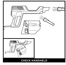
Remove the handheld vacuum from the wand and check all dust cup intake openings.
