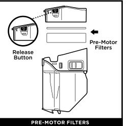
To access the pre-motor filters, press and pull both filter access tabs on the dust cup to remove the filter holder. The **Pre-Motor** Filters should be washed twice a month.
