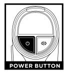
Press the power button to begin vacuuming. To turn off power, press button again.
