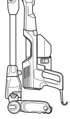
Looking at the vacuum from the side with the cord hooks, wrap the power cord anti-clockwise around the hooks, starting under the bottom hook. Then press the Flexology Wand Lock Release button and gently fold the handheld vacuum forward toward the floor nozzle.
